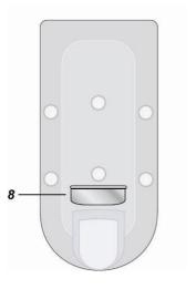
When the tamper switch is compressed, Factory Reset of the PIR Camera is disabled.
