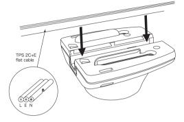
Place the cover on top of the main body and press the pins firmly into the guides.
