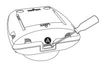
Slide the cover back until you can remove it completely.
