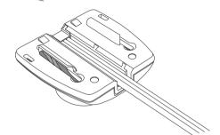
Place the cover on top of the main body and press the pins firmly into the guides.
