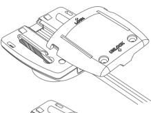
Slide the cover closed until you hear a 'click' sound for a safe and secure termination.
