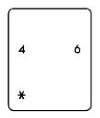
When all buttons on the keypad are displayed, enter your password (4~12 digits) and then press [\*] to open the door.
