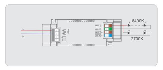
Installation: light driver is packed in white paper box wripped with black metal ceiling cap, connect the brown wire to LED+, Blue wire to LED W and White Wire to LED C.
